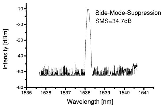
Fig. 4. Spectrum of the DBR laser with a side mode suppression of 34.7 dB.
