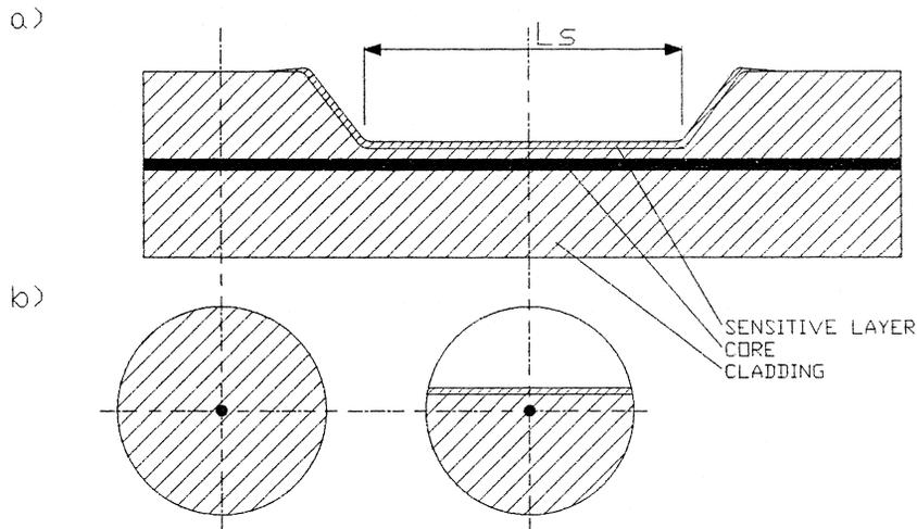
Fig. 1. Section of the cavity with the sensitive element: (a) longitudinal cut, (b) cross cut (unpolished fiber and after polishing and coating).
