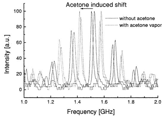
Fig. 5. The presence of acetone vapor induces a shift in the output frequency of the DBR laser. This figure shows four snapshots of the spectrum, two with and two without acetone vapor.
