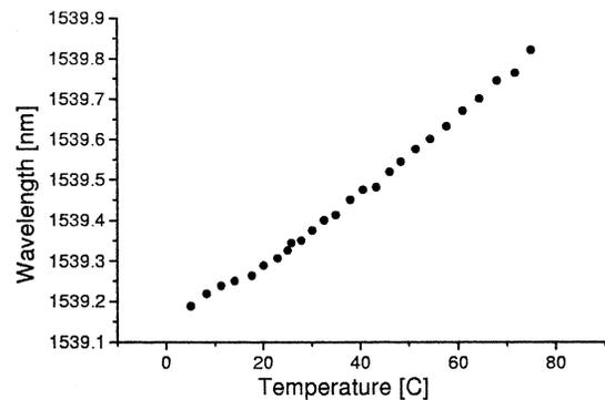
Fig. 6. Oscillation frequency of the DBR laser for varying temperature.
