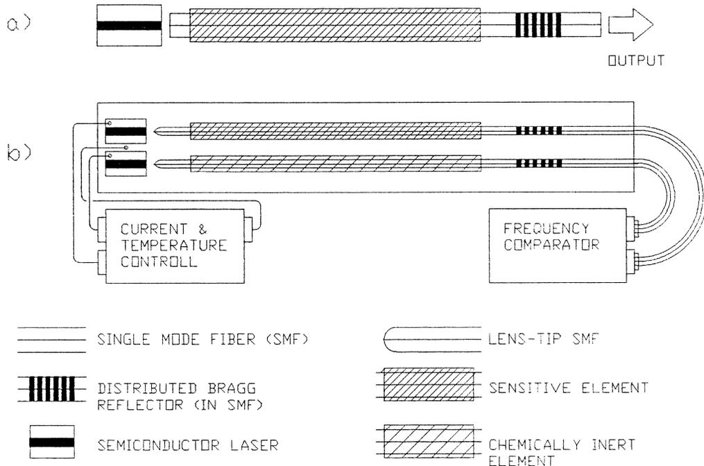
Fig. 2. (a) Single line sensor. (b) Two-line set-up using heterodyne detection.
