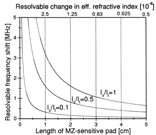
Fig. 3. For certain ratios of  $l_s/l_t$  the expected resolution is plotted. The resolvable change in effective refractive index is compared to a Mach–Zehnder-based sensor of varying length. Here we assumed a resolvable phase shift of  $1 \times 10^{-3}$  rad.
