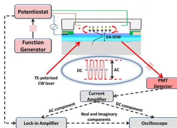
**Fig. 2.** Experimental setup includes a potentiostat for electrical control of the EA-IOW interface, laser light source, photo-multiplier detector, current amplifier, lock-in amplifier, and an oscilloscope for data collection.
