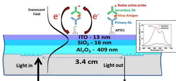
**Fig. 1.** Structure of the multilayer, single-mode EA-IOW device functionalized with a sandwich bioassay: an APTES monolayer, covalently bounded primary (capture) antibody, virus protein (antigen), and secondary antibody conjugated with the methylene blue redox-active optical probe. Inset: spectral molar absorptivity of methylene blue after conjugation with the secondary antibody at different oxidation states.
