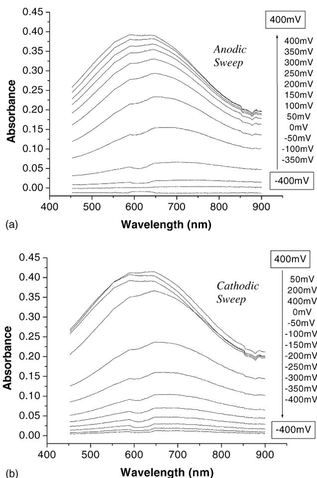
Fig. 3. ATR spectra of a self-assembled PANI/PAA/PANI/PAA film in contact with 0.1 M, pH 7.0 phosphate buffer, acquired during oxidation (a) and reduction (b) at 50 mV intervals between  $-400$  and  $400$  mV. The scan rate was 5 mV/s. Due to the similarity and overlap of spectra near the positive and negative limits of the potential range, not all spectra are shown.
