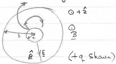
Two conducting cylinders, co-axial with an  $E$  field between them.
