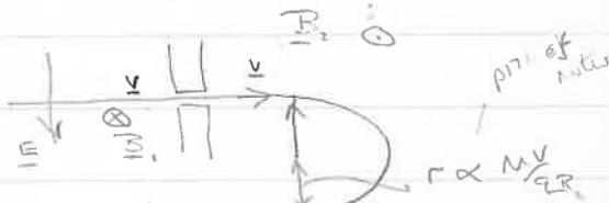
This is the principle of the mass spectrometer.
