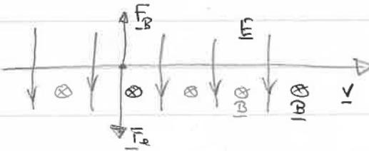
If the particle moves with velocity  $v$  at right angles to  $E$  and  $B$ . Then there will be no
