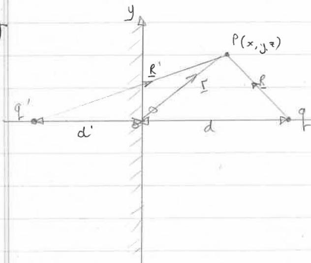
$$\begin{aligned}\underline{r} &= \hat{x}x + \hat{y}y + \hat{z}z \\ \underline{r}' &= \hat{x}d \\ +x &\quad -r' = -\hat{x}d'\end{aligned}$$
