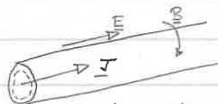
For time varying currents (a.c.) this is equivalent to the passage of an EM wave, of the same frequency as the ac, into the conductor. But we have just shown that in such a case the EM field is restricted to the skin-depth ( $\delta$ ). Thus the current flows only in a thin region close to the surface.
