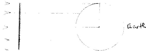
Since the earth is so far from the sun we can safely assume that the radiation from the sun forms a parallel beam as shown above.
