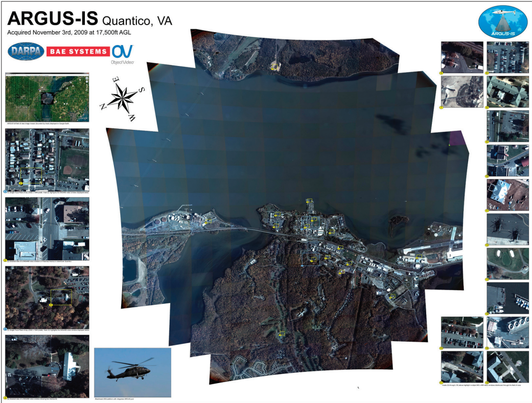
FIGURE 4.2 A sample of the ARGUS-IS imagery. The system was mounted under a YEH-60B helicopter flying at 17,500 feet over Quantico, Va. The Argus-IS images an area more than 4 km wide. The ARGUS system uses a large number of inexpensive cell phone cameras to create a whole new imaging modality with a huge format. SOURCE: Image available from DARPA Information Innovation Office, Autonomous Real-time Ground Ubiquitous Surveillance-Imaging System (ARGUS-IS), at http://www.darpa.mil/Our_Work/I2O/Programs/Autonomous_Real-time_Ground_Ubiquitous_Surveillance-Imaging_System_%28ARGUS-IS%29.aspx .
