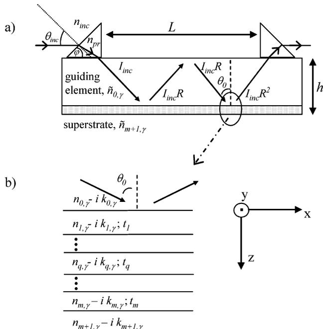
**Figure 1.** (a) ATR configuration showing the path of the light beam as it is incoupled, reflected down the ATR substrate, and outcoupled. (b) Expanded view of the multilayer structure showing our coordinate system where the  $x$ - $y$  plane is the sample plane and light is propagating in the  $x$ - $z$  plane.
