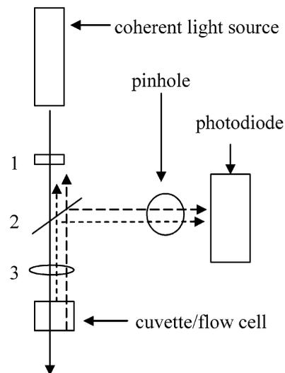
**Figure 3.** Interferometer setup: (1) lens to expand beam; (2) beam splitter (glass slide); (3) iris. The solid line is the incident beam and the dashed lines are the beams reflected from the front and back glass/air interfaces of the cuvette.
