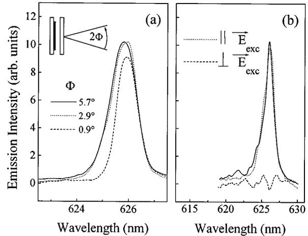
**Fig. 7** (a) Detected planar cavity emission spectrum above the laser threshold for various apex angles  $\Phi$  of the detection cone, indicating nearly diffraction-limited laser output. (b) Emission spectrum of the laser cavity detected without analyzer (solid line, normalized), with an analyzer parallel to the exciting laser (dotted line), and with an analyzer perpendicular to the exciting laser (dashed line), showing a polarization degree better than 50 : 1.
