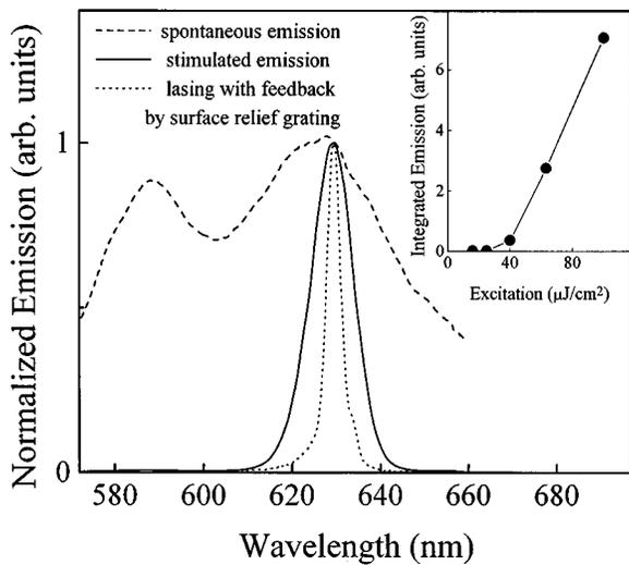
**Fig. 8** Comparison of the emission spectra from a 200-nm BEH:PPV film: Spontaneous emission at low excitation (dashed line), stimulated emission without feedback (solid line), and laser emission with feedback provided by a surface relief grating (dotted line,  $\Lambda=500$  nm). Inset: Integrated emission intensity of the laser structure as a function of excitation.
