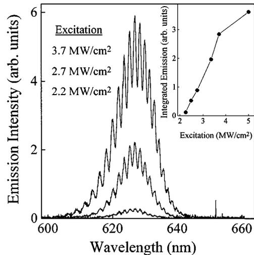
**Fig. 10** Emission spectra of a waveguide ring resonator structure covered with a 200-nm BEH:PPV film for different excitation levels of the polymer layer. The spectra are observed at the output of a channel waveguide that is slightly coupled to the ring resonator. Inset: Spectrally integrated output of the straight waveguide as a function of optical excitation of the polymer film. The emission has been normalized to the excitation fluence.
