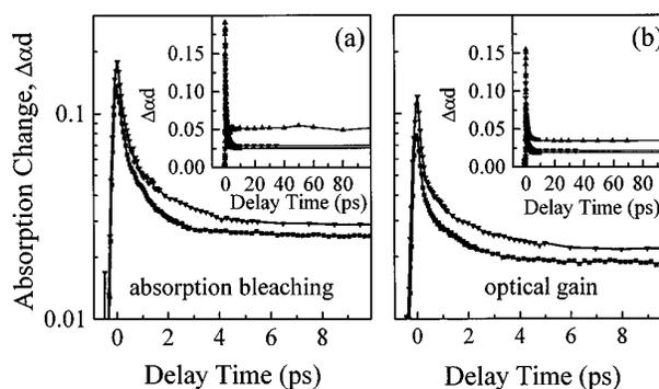
**Fig. 5** Decay curves of the excitation-induced absorption change at two different wavelength representing (a) absorption bleaching at 575 nm and (b) optical gain at 621 nm. Data for excitation fluences of  $100 \mu\text{J}/\text{cm}^2$  (squares),  $150 \mu\text{J}/\text{cm}^2$  (point-down triangles), and  $400 \mu\text{J}/\text{cm}^2$  (point-up triangles) are plotted. The insets show the same signals on a longer time scale.
