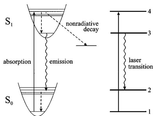
**Fig. 1** Schematic drawing of the energy-level diagram of an organic material (left) and the corresponding approximate four-level picture (right).
