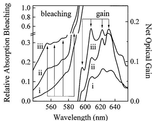
**Fig. 3** Relative absorption bleaching  $-\Delta\alpha/\alpha_{\text{lin}}$  (left) and net optical gain  $(-\Delta\alpha - \alpha_{\text{lin}})d$  (right) measured in the absorbing and the transparent regions of a 190-nm BEH:PPV film, respectively. The data for three different pump pulse fluences (i: 100, ii: 400, iii:  $1000 \mu\text{J}/\text{cm}^2$ ) are taken at zero delay between pump and probe pulses. Arrows indicate the transition energies in absorption and stimulated emission.
