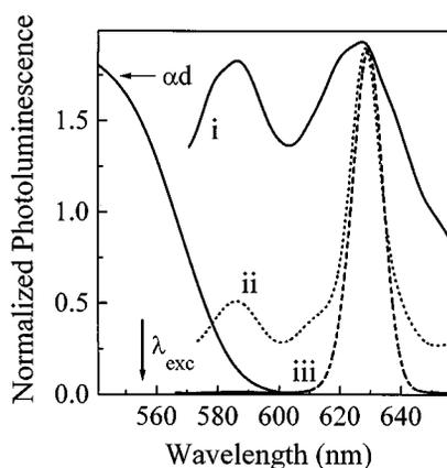
**Fig. 2** Normalized PL spectra of a  $100\text{-nm}$  BEH:PPV film after excitation with  $100\text{-fs}$  pulses ( $\lambda_{exc} = 555\text{ nm}$ ) and excitation fluences of (i)  $30$ , (ii)  $50$ , and (iii)  $120\text{ }\mu\text{J}/\text{cm}^2$ . For comparison the absorption spectrum is also given.
