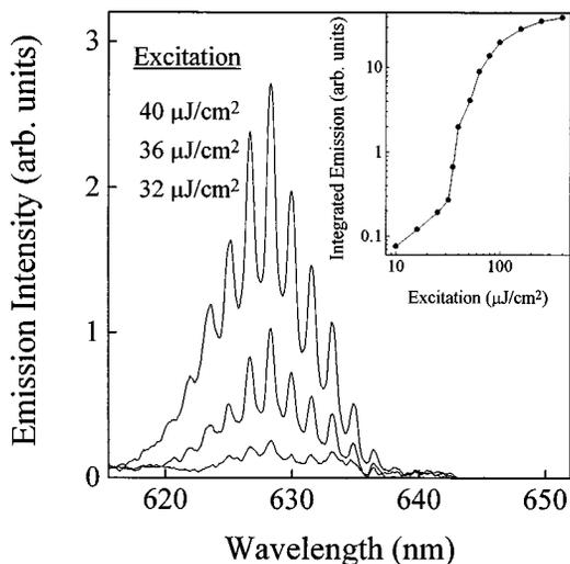
**Fig. 9** Emission spectra from a polymer microring encircling an optical fiber of 56- $\mu\text{m}$  diameter at three different excitation intensities. Lasing of whispering-gallery modes is found for excitation above  $30 \mu\text{J}/\text{cm}^2$ . Inset: Integrated emission intensity as a function of excitation.
