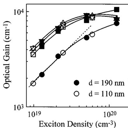
**Fig. 4** Dependence of the optical gain coefficients ( $\Delta t=0$ ) on the excited exciton density. The gain at four different wavelengths is plotted: point-up triangles: 630 nm; point-down triangles: 621 nm; squares: 609 nm; circles: 595 nm. Open and closed symbols are measured at a 110-nm film and a 190-nm film, respectively.
