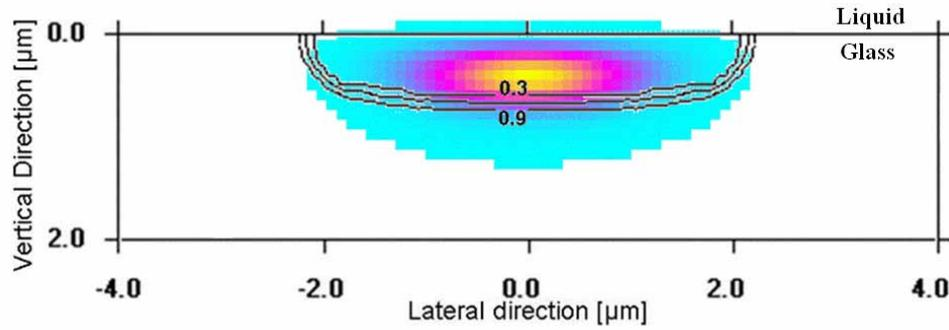
Fig. 2. The silver ion concentration and fundamental mode intensity profile (the solid contour lines are for normalized concentrations of 0.3 0.6 and 0.9 and colors from blue to yellow are for increasing intensity).
