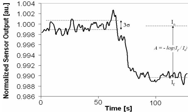
Fig. 5. Response of the sensor to 1 nM of cyt c solution. This corresponds to about 270  $\text{pg}/\text{cm}^2$  surface coverage. The signal change is  $I_0 - I_f \approx 0.01$ , which in absorbance units corresponds to  $A = -\log(0.99) \approx 4 \times 10^{-3}$ , well above than the  $A_{\text{LOD}} = 8.69 \times 10^{-4}$ .
