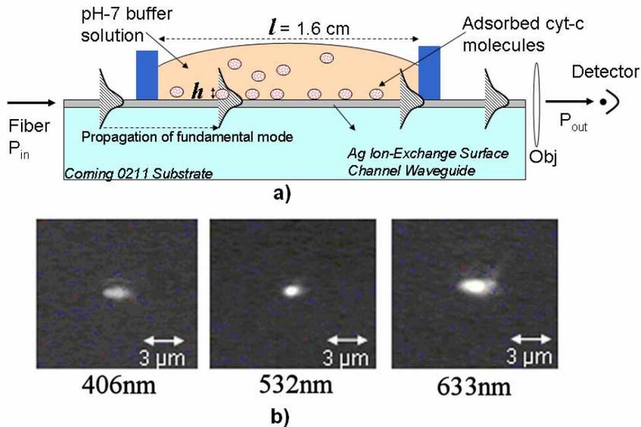
Fig. 1. (a). The schematic of the waveguide sensing platform. The fundamental mode of Ag ion exchange waveguide interacts with the surface adsorbed cyt c molecules for a pathlength of  $l = 1.6$  cm. Interaction strength,  $\kappa$ , is determined by  $h$  and evanescent tail of the mode as shown. (b) Near field images of the waveguide output. Only the fundamental mode was excited at 532 nm. Superposition of two lateral modes can be seen for 406 nm.
