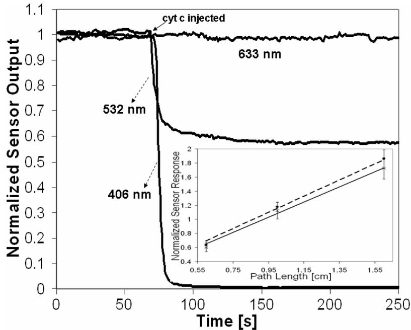
Fig. 3. Experimental data showing the response of the sensor to about one half of a monolayer of cyt c. The inset shows the normalized sensor response ( $A/(\epsilon \kappa)$ ) with respect to the probing path length at 406 nm (dashed line) and at 532 nm (solid line). The SNR is measured to be  $\sim 1500$  for 406 nm laser source.
