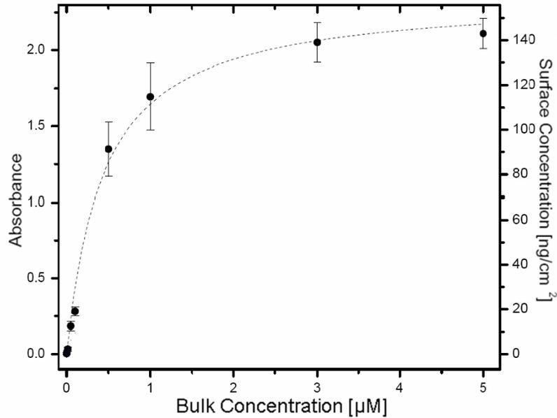
Fig. 4. Adsorption isotherm of cyt c on the glass surface at pH-7, measured at 406 nm. The dashed curve is the best fit of the experimental data to a Langmuir adsorption model with  $K_a = 2.4 \times 10^6 \text{ M}^{-1}$ . The error bars are showing the surface concentration variance of independent three measurements.
