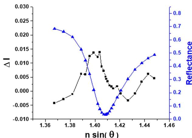
**Fig. 3.** Right  $y$  axis shows the SPR reflectance for the buffer solution, while the left  $y$  axis shows the difference in the optical signal  $\Delta I$  between the oxidized state and the reduced state of the MB molecule.
