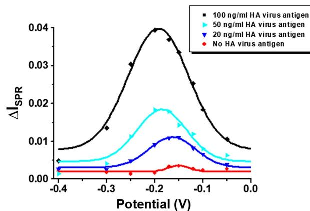
**Fig. 6.** SPR optical signal  $\Delta I_{\text{SPR}}$  versus the DC bias potential in the absence of HA virus antigen and for different concentrations of the HA virus antigen measured under a sinusoidal potential modulation at the frequency of 250 Hz and an amplitude modulation of 0.04 V.
