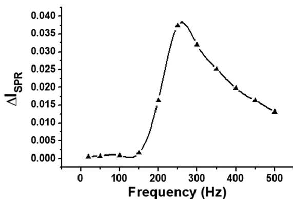
**Fig. 5.** SPR optical signal  $\Delta I_{\text{SPR}}$  measured under AC potential modulation at the DC bias potential of  $-0.17$  V and a HA virus antigen concentration of 200 ng/ml.
