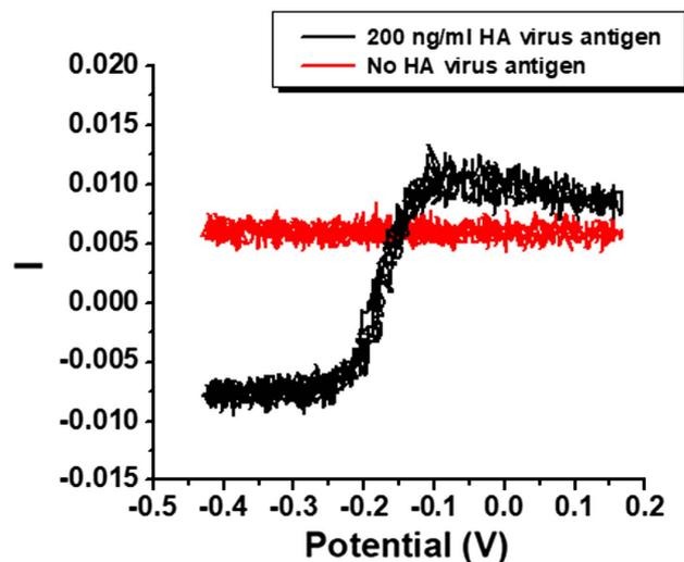
**Fig. 4.** Optical signal  $I$  under a CV scan for the full immunoassay sandwich at scan rate of  $0.02$  V/s. The red trace shows the data in the absence of HA virus antigen, while the black trace represents the data in the presence of HA virus antigen.
