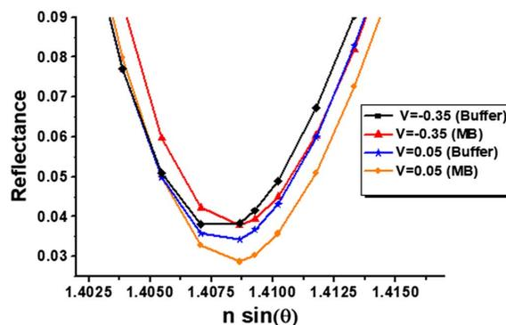
**Fig. 2.** SPR reflectance for the PBS buffer and MB solutions at  $-0.35$  V and 0.05 V.
