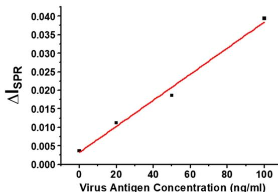
**Fig. 7.** Calibration curve based on AC measurements for detection of different concentrations of the HA virus antigen.
